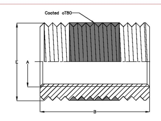
Female thread A = M6Length B= 15Male thread E= M8Type= 97x 000 060.100
